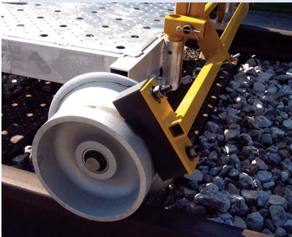
▲ ATS cart showing close-up of Nolan's coaster brake system
